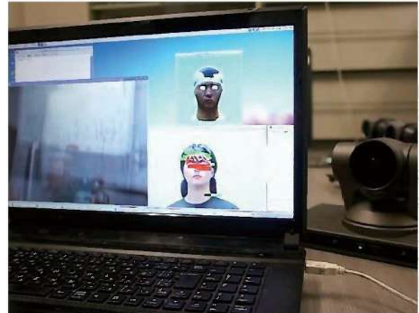
A remote vision system with a three-dimensional vision interface and a vision robot with eye movement capability
