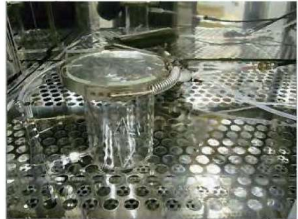
The measurement of SVOC emission rates from PVC sheets using a micro-chamber.
