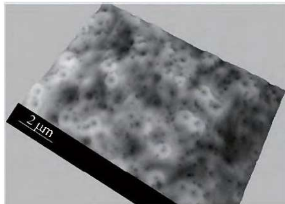
Direct observation of nanoscopic emission distribution of InGaN semiconductor alloy by Cathodoluminescence mapping
