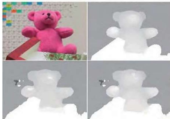
Figures: an image captured by a left-side camera (upper left), the ground truth of the distance map (upper right), distance maps computed by a conventional method (lower left), and our method (lower right).
