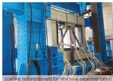
Loading test equipment for structural experimentation
