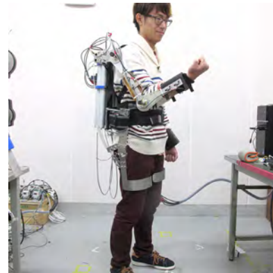
The 2nd prototype of our powered exoskeleton driven by McKibben artificial muscle
