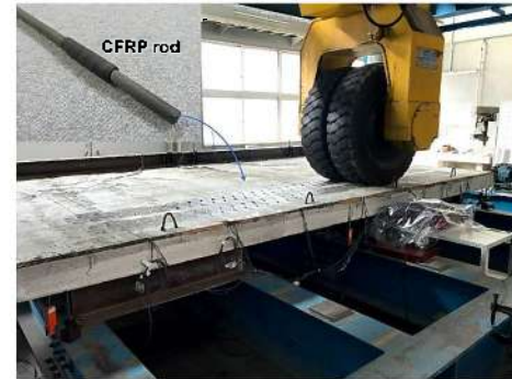
Moving-wheel load test for a cantilever RC slab strengthened with CFRP rods
