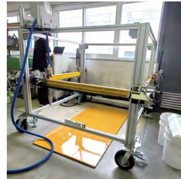
A 3D printer used for construction. The nozzle moves around the area enclosed by the frame to eject the mortar that will be used as ink.
