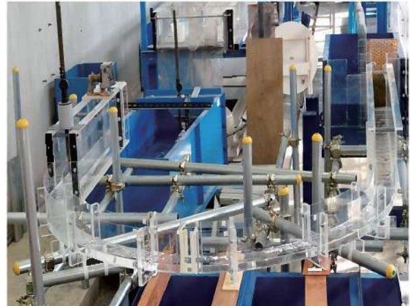
Experimental setup for study on lateral overflow in curved open channels
