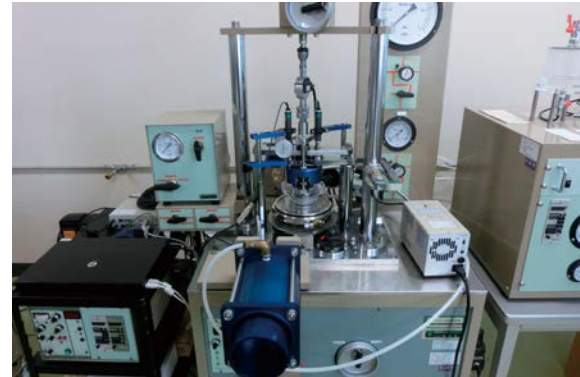
The "Cyclic ring shear test apparatus" we developed. It has the smallest specimen among similar test apparatuses (inner dia. 42mm, outer dia. 70mm, height 20mm). Shear and normal forces, skin frictional force, shear and normal displacements, pore water pressure are severally monitored. It provides the macro zoom capture system for observation of soil particles around slip surfaces.
