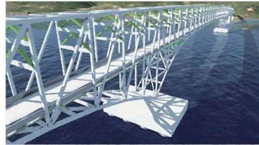
Three-dimensional model of a bridge structure (digital twin) created for conducting simulations of bridge earthquakes
