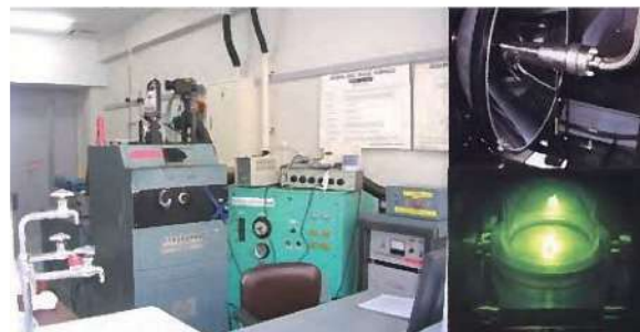
Xenon arc image furnace. A simulated solar furnace capable of attaining maximum temperatures of over 3000°C
