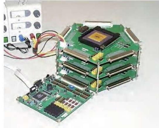
Prototype of a self-reconfigurable parallel system
