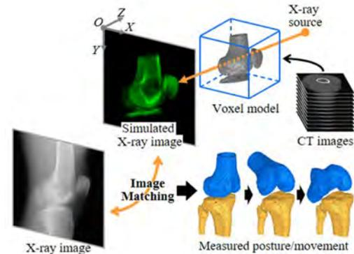
*In vivo* joint kinematics is measured with model-image registration methods that use medical images
