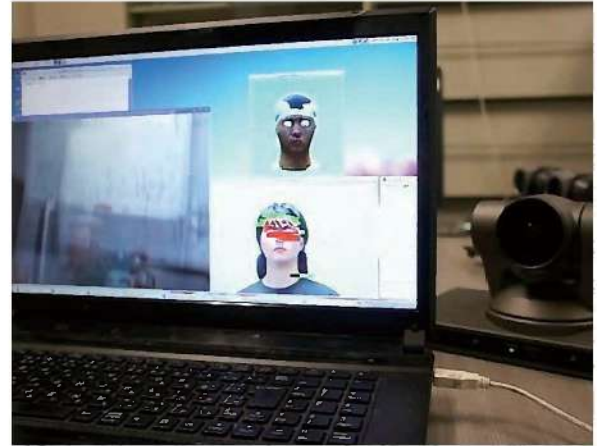
A remote vision system with a three-dimensional vision interface and a vision robot with eye movement capability
