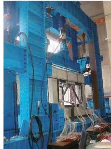
Laboratory equipment and 1:2.5 scale reinforced concrete frame specimen retrofitted with steel braces
