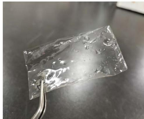
Ammonium-selective ion exchange membrane under development
