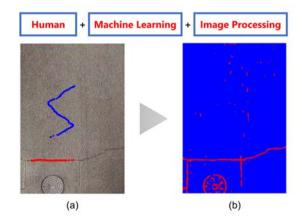
Example of "interactive image processing": training of crack detection model, and result of crack detection using trained model.
