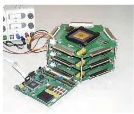
Prototype of a self-reconfigurable parallel system
