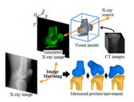
*In vivo* joint kinematics is measured with model-image registration methods that use medical images
