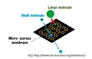
Molecule sieving by means of a micro-porous membrane
