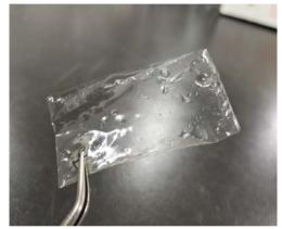
Ammonium-selective ion exchange membrane under development
