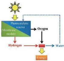
An application of membrane gas separation to photocatalytic hydrogen production
