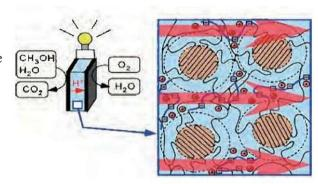
Schematic image of a direct methanol fuel cell and polymer electrolyte membrane having ion paths by nano-phase separation
