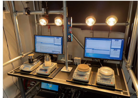
Measurement of the geotechnical properties of unsaturated soil using the developed laboratory test method.
