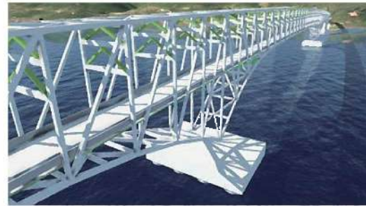
Three-dimensional model of a bridge structure (digital twin) created for conducting simulations of bridge earthquakes
