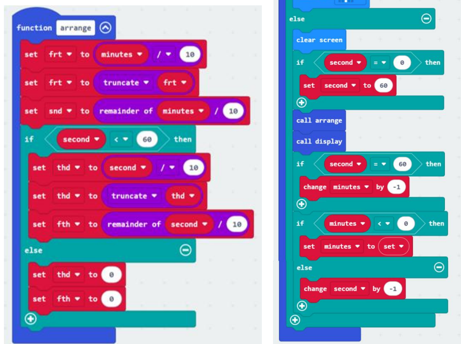
Code 7. Program for countdown (calculation processing: MakeCode)
