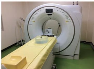
YUAMEC is equipped with a 64-row helical-computed tomography (CT) , which can obtain detailed imaging information of dogs and cats in a short time and is useful to diagnose diseases and determine the underlying pathogenesis.
